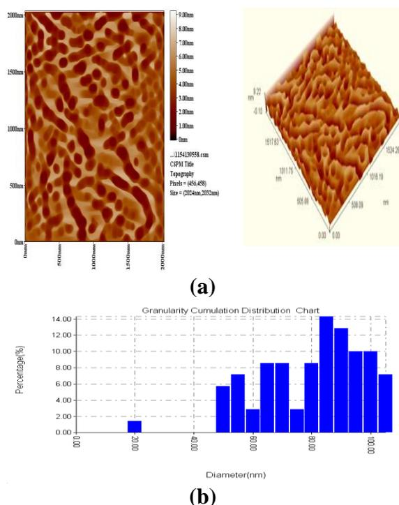
**Fig.(9):(a) 2D, 3D AFM image, (b) granularity accumulation distribution of porous silicon prepared at 532nm wavelength green laser with power 30 mW, etching time 3 min and current 10 mA at 25% HF concentration.**
