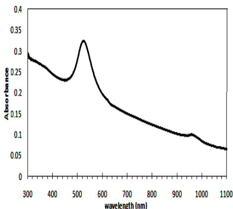
**Fig.(3): Absorption spectrum as a function of wavelength of Au nanoparticles synthesis by laser ablation in DIW.**
