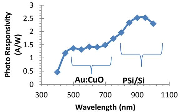
**Fig.(14): Responsivity as function of wavelength for Au:CuO/ porous silicon heterojunction at reverse bias voltage of -2.5 Volt.**
