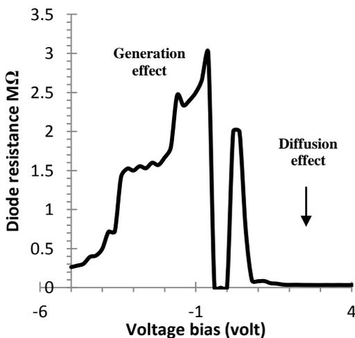
Fig.(11): The variation of diode resistance via voltage bias in the dark current.
