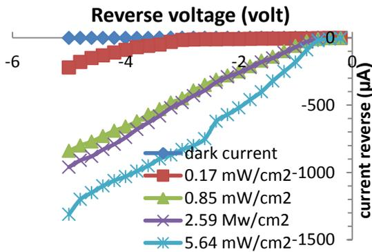
**Fig.(13): Current-voltage in reverse bias of Au:CuO/porous silicon heterojunction under illumination with different intensity of the light.**
