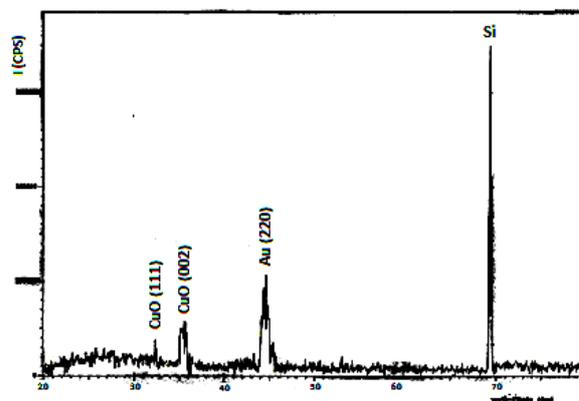
**Fig.(8): X-Ray Diffraction pattern of Au:CuO nanocomposite synthesis by laser soldering in DIW deposited on porous silicon.**
