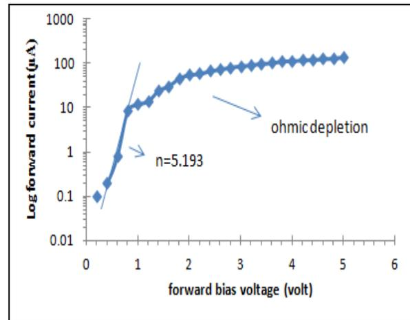
Fig.(12): Semi-log current–voltage characteristic in forward bias.
