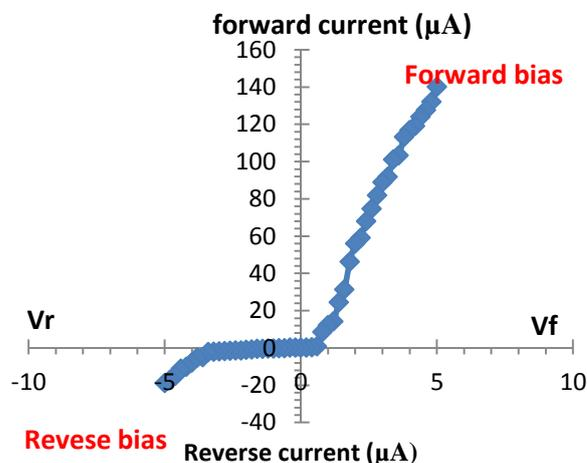
**Fig.(10): Current-voltage in forward and reverse bias of Au:CuO nanocomposite/ porous silicon hetrojunction in the dark at room temperature.**
