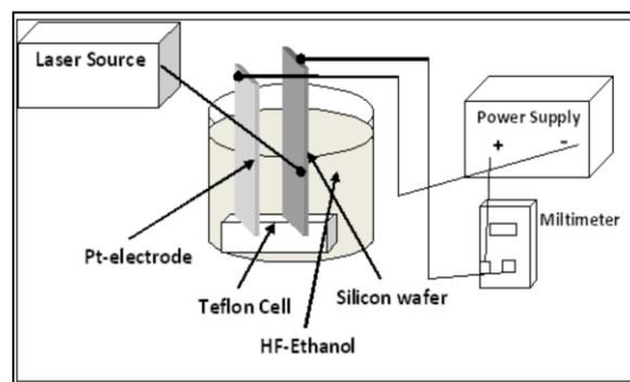
**Fig.(2): Schematic diagram of photo chemical method.**
