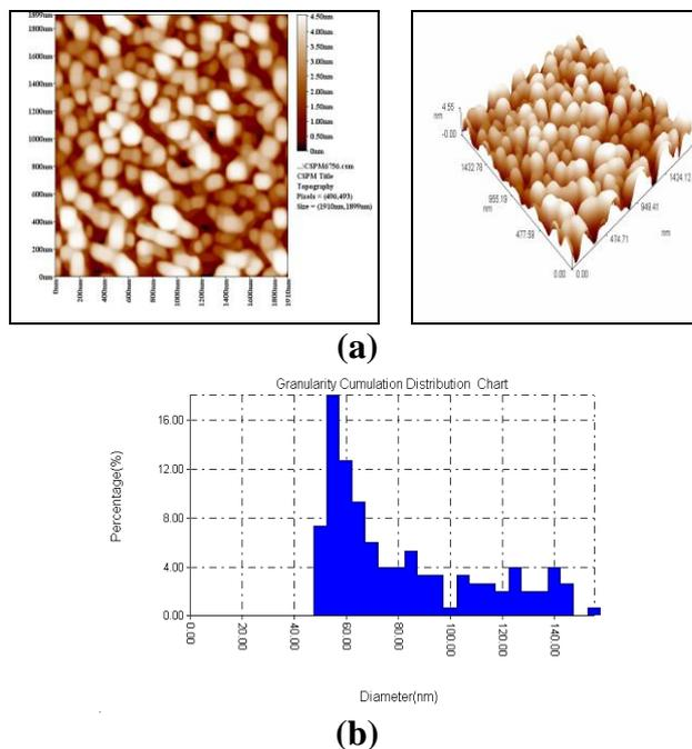
**Fig.(7): (a) 2D, 3D AFM image, (b) granularity accumulation distribution of Au:CuO nanocomposite synthesis by laser soldering in DIW.**
