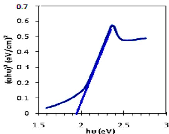
*Fig.(5): (a) The absorption spectrum of Au:CuO nanoparticles, (b) band gap of Au:CuO nanoparticles synthesis by laser soldering in DIW.*
