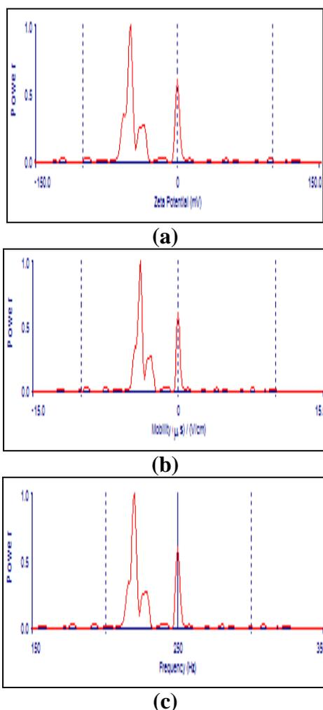
**Fig.(6): (a) The zeta potential, (b) the mobility and (c) the frequency shift of Au:CuO nanocolloidal synthesis by laser soldering in DIW.**
