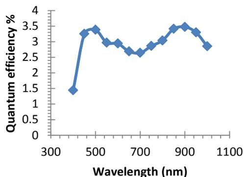
**Fig.(15): Quantum efficiency as function of wavelength for Au:CuO/ porous silicon heterojunction at reverse bias voltage of -2.5 Volt.**
